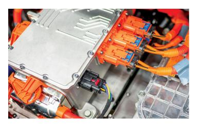
Tests in the field showed no change in electrical conductivity, as well as consistent friction values over 250+ mating cycles, when MOLYKOTE® L-8030 Semi-Dry Lubricant was used.
