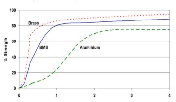
Cure times are typical at 23°C. Copper and its alloys will follow the faster cure while oxidised or passivated surfaces like stainless steel will tend towards the slower curve. Lower temperatures or large gaps will tend to extend the cure time. To reduce the cure time the use of Permabond A905, ASC10, or heat can be considered.
