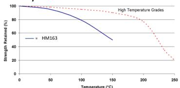
"Hot strength" shear strength test's performed on mild steel. 24hr cure at room temperature and conditioned to pull temperature for 30 minutes before testing.
