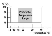
Any combination of the above conditions will ensure a cure schedule sufficient to allow transportation of the glazed modules within 21 days, depending on joint configuration. Consult technical services for specific advice.
