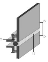
**<u>Figure 5</u>**: Design with stepped insulating glass unit.
