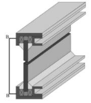
**<u>Figure 3A</u>:** Transom detail. Examples of structural glazing designs: 4-sided design (factory glazed).
