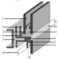
**<u>Figure 2A</u>:** Transom detail. Examples of structural glazing designs: 2-sided design (installed on site).
